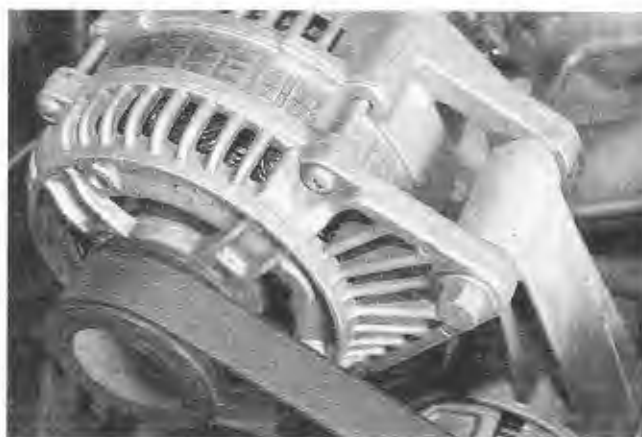
13.4b ... as well as the mounting bolts
