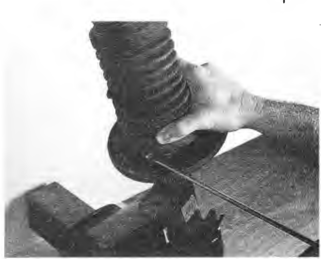
8.14a Loosen the dust boot clamp with a screwdriver ...
