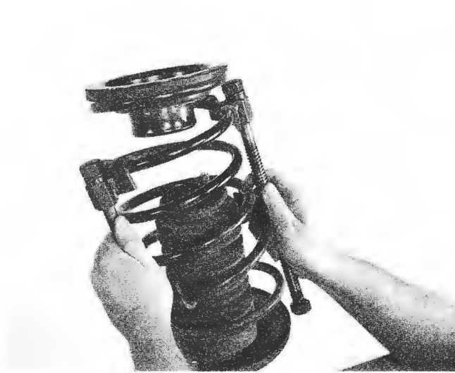
8.9 The spring and compressors can be lifted off the assembly
