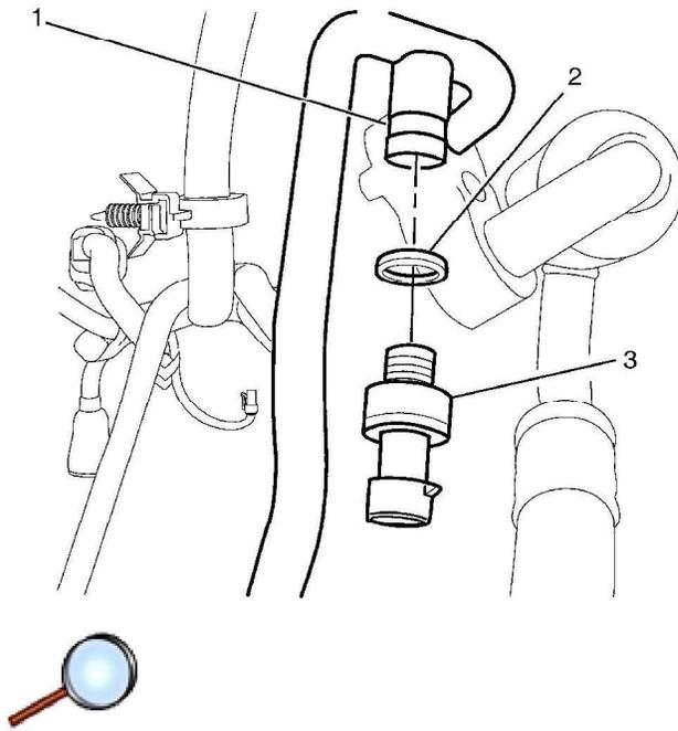
**Important:** A Schrader valve is fitted to the A/C refrigerant pressure sensor port (1). Upon removal of the A/C refrigerant pressure sensor (3) you will, for a very short period, hear refrigerant escape until the Schrader valve reseats. If refrigerant continues to escape while removing the A/C refrigerant pressure sensor (3) STOP IMMEDIATELY. The Schrader valve has a fault and the refrigerant will have to be recovered.
