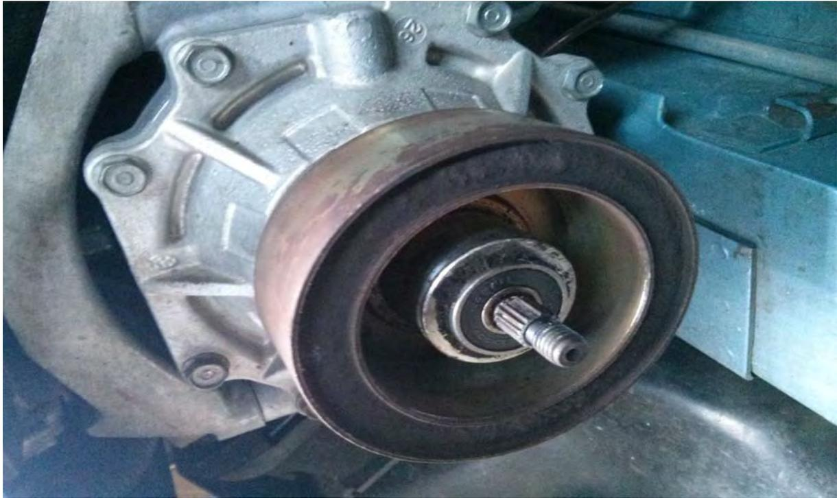
12. Reinstall the circlip onto the front of the compressor.
