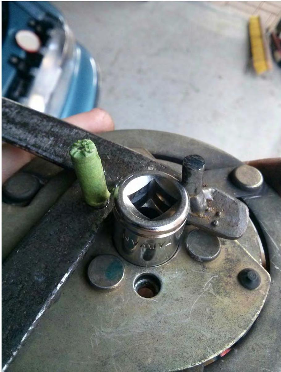
4. Remove the clutch, I got it off with a bit of wiggling, some penetrating oil might help too. Be careful of the shims (thin washers) falling out.
