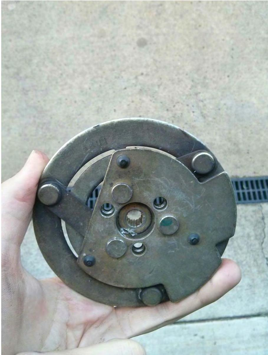
5. Remove shims and put in a safe place, mine had two shims; the number will vary from car to car.
