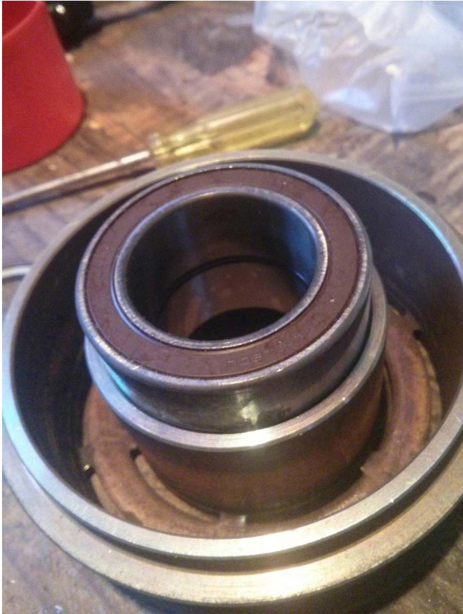
10. Reinstall circlip.
