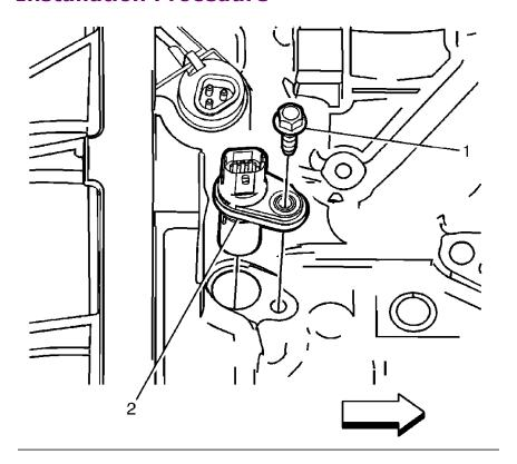
1. Install the CKP sensor (2) to the engine block.
