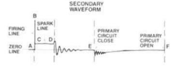
at right in position A to B). This represents the voltage required to overcome the spark plug and distributor rotor gaps. Once the spark gaps have been bridged, the secondary voltage required to sustain the spark across the gap is much less and drops (as seen in position B to
