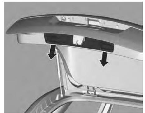
Use the handle to pull down the tailgate until it drops under its own weight. The tailgate closes and latches itself automatically.
